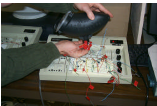
FIGURE. 2 ELECTRONICS FOR PAINTBALL HOPPER SYSTEM. ALONG WITH A PART OF CASING.
