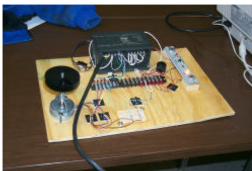
FIGURE. 7 PROTOTYPE OF THE AUTOMATIC PILL DISPENSING SYSTEM.
