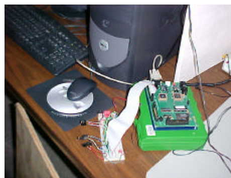
FIGURE. 6 ELECTRONICS DESIGNED FOR MOTORCYCLE GEAR DETECTION SYSTEM.
