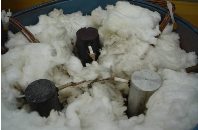
FIGURE 1 INSTRUMENTED METAL BARS WITH INSULATION
