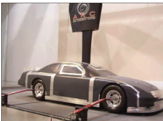
FIGURE IV AERODYNAMIC TESTING OF A 40% SCALE MODEL RACECAR AT THE AUTO RESEARCH CENTER (ARC) IN MOORESVILLE, NC.
