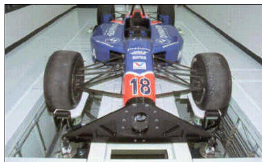
FIGURE V SEVEN-POST VEHICLE DYNAMICS RIG AT THE AUTO RESEARCH CENTER (ARC) IN INDIANAPOLIS, IN.
