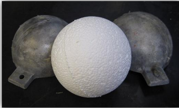
Figure 1: 3.0" diameter expandable foam bead ball with mold halves
