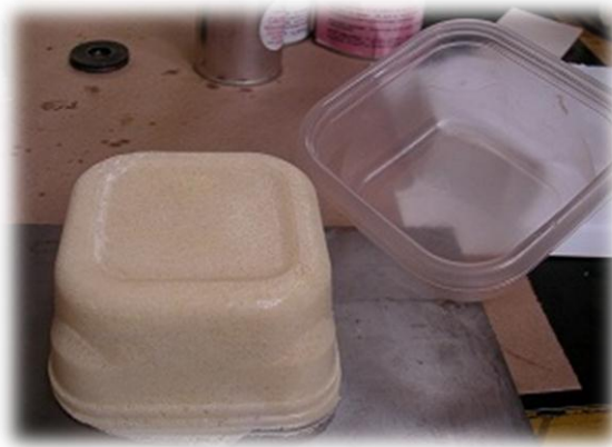
Figure 2: Chemical foam block with its disposable plastic mold
