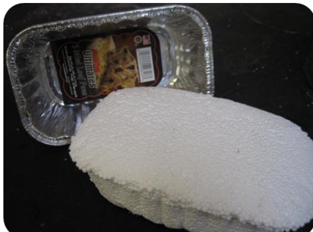
Figure 3: Expandable foam bar and part of mold, prior to cutting to test size
