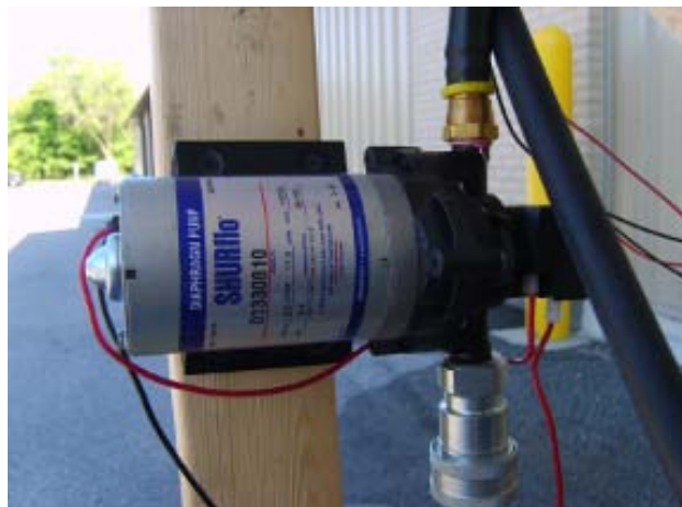
Figure 2: Close-up view of the water pump
