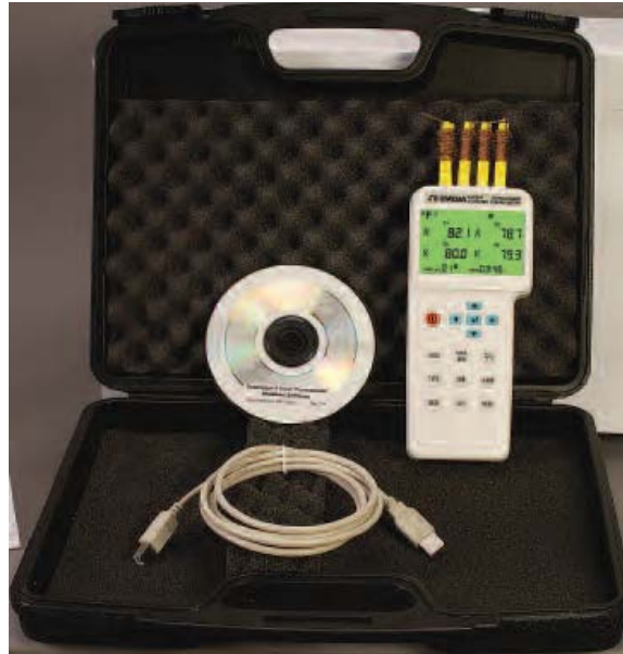
Figure 6: HH1384 data logger 4-input thermometer
