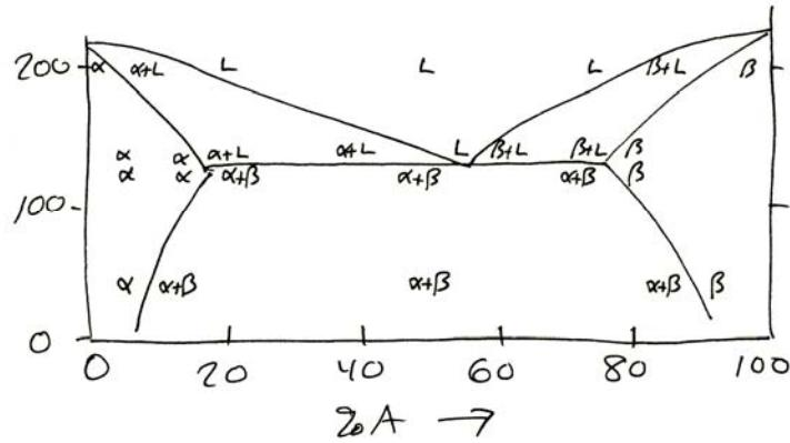
Figure 13: Typical hand-drawn phase diagram created from the data in Table 2.
