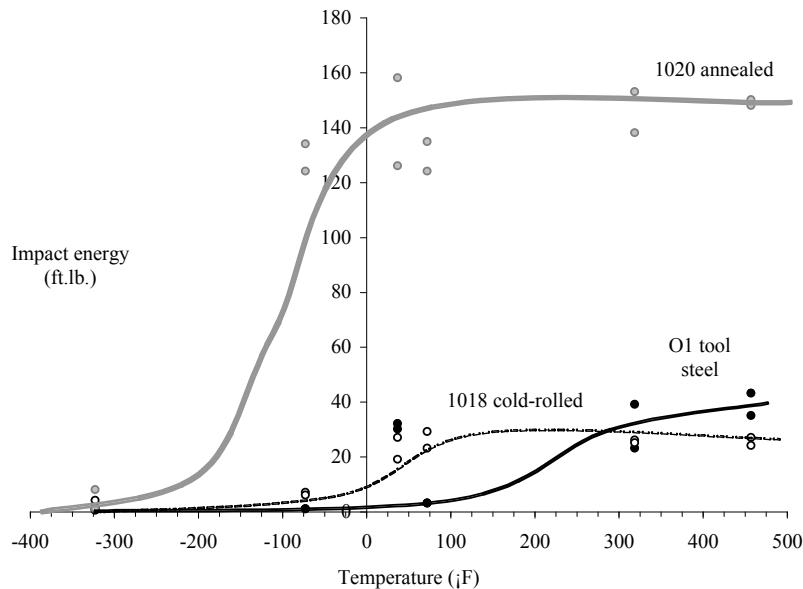
Figure 11: Typical results from an impact test of three materials. O-1 tool steel shows the strangest behavior: impact energy around 35 ft.lb. in icewater, and below 5 ft.lb. at room temperature. Students learn that samples are sometimes mislabeled.
