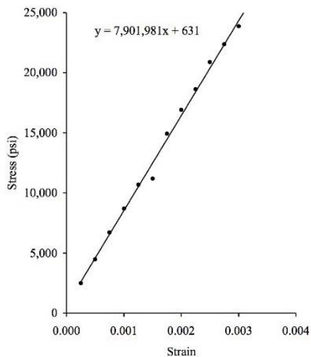
Young's modulus is the slope of the elastic portion of the stress-strain curve. One way to find it is to plot only the elastic stress/strain data on an x-y graph, and use linear regression (select **Add Trendline** from the chart menu in MS Excel). This graph uses only the first 12 data points...after that, the material permanently deforms. Under **Options**, display the equation, then change the number format if needed.
