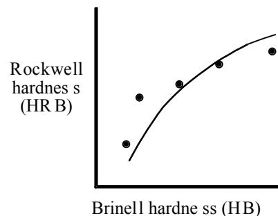
Figure 2: Improved diagram of a hardness plot from the Spring 2007 laboratory manual, showing the ASTM least-squares curve.
