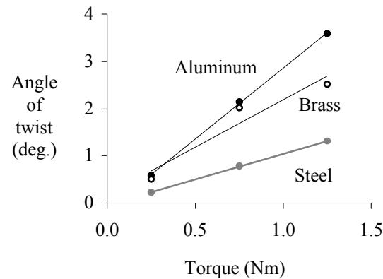
Figure 5: Data from Figure 4. Straight-line linear regression lines suggest that the middle reading for brass is high, and that the slope is less than aluminum, which is consistent with published values of shear modulus.
