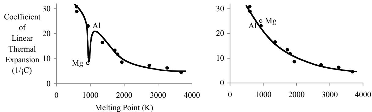
Figure 12: At left, a typical student homework submission shows magnesium substantially below the trendline. Many students draw a line passing through the magnesium point. When the correct value of magnesium is used (right), the trendline passes near all points.
