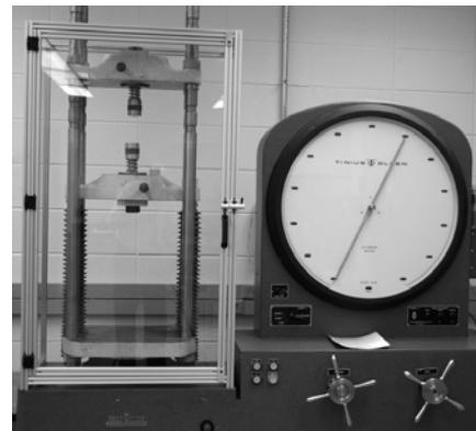
Figure 6: Old-style hydraulic tensile testing machine.
