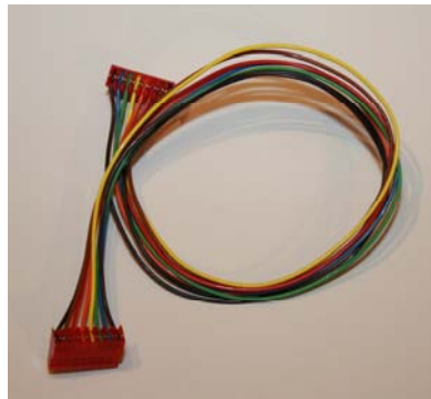
Figure 7 – Typical Microcontroller Interface Cable
