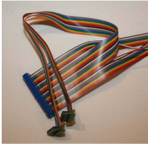
Figure 9 – Altera DE1 Interface Cable
