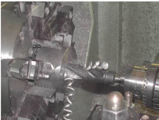
Figure 10 – Boring the Slider Center Hole
