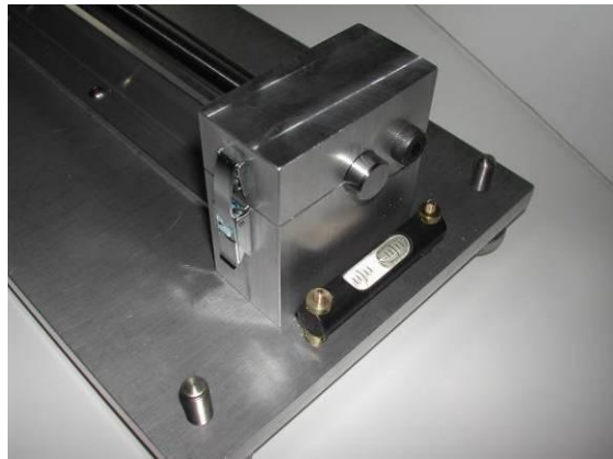
Figure 9 – Completed and Installed End Clamp
