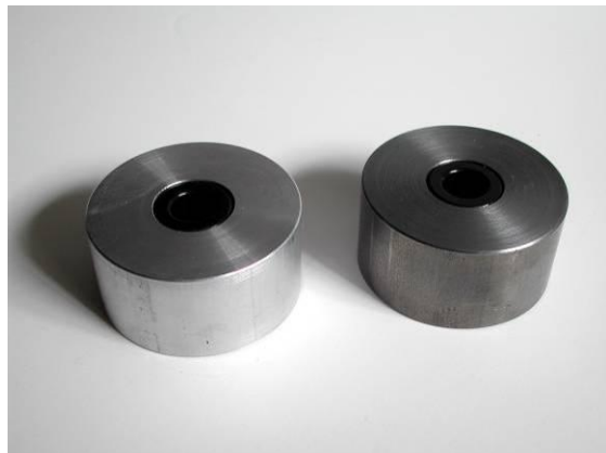
Figure 11 – Completed Aluminum and Steel Sliders
