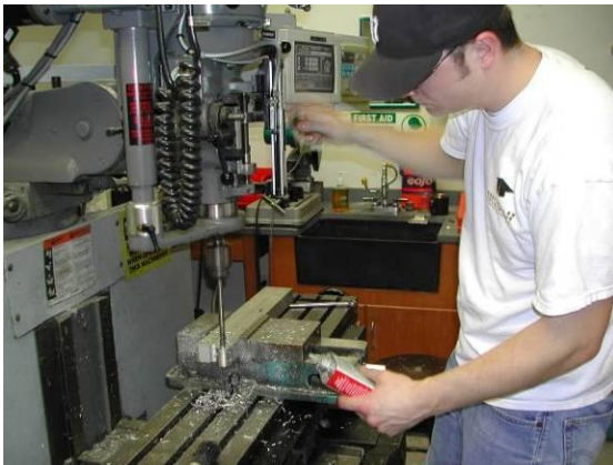
Figure 8 – Boring a Hole
