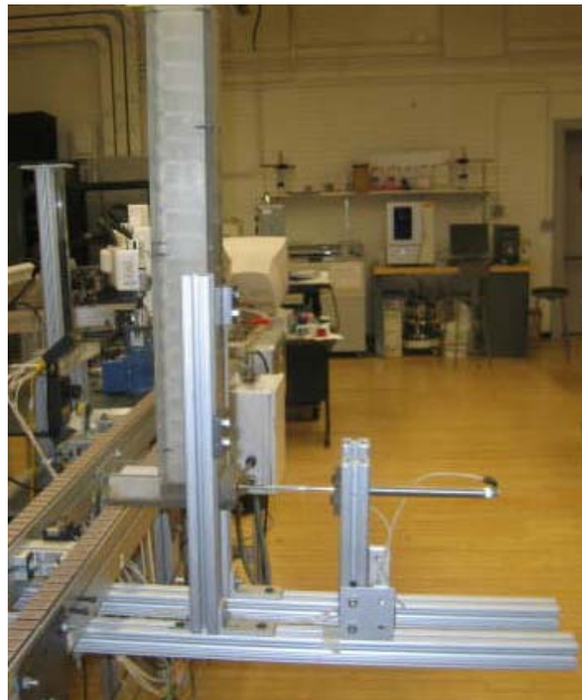
Figure 4. The re-designed bottle feeding rack.
