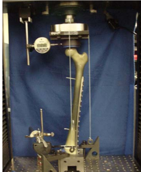
Figure 2. Test setup to determine stiffness and gap strain in bone plates
