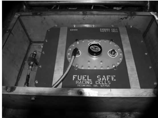
Figure 6 – Installation of the fuel system in the IUPUI racecar.
