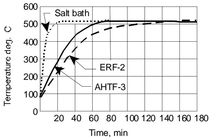
**Figure 4. Heating curve of metal from the moment of loading of the furnace to the temperature of 515°C for bars and forgings 100 mm thick weighing 160 kg.**
