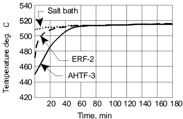
**Figure 3. Heating curve of metal from the moment of loading of the furnace to the temperature of 515°C for bars and forgings weighing 160 kg.**
