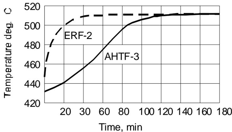
**Figure 2. Heating curve of metal from the moment of loading of the furnace to the temperature of 515°C for bars and forgings weighing 350 kg.**
