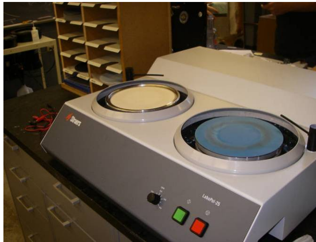
Figure 3.2: Photograph of Struers Labopol-25 Polishing Wheels used to obtain a mirrored finish. These wheels are capable of angular velocities from 0 rpm to 500 rpm and support both magnetic mount as well as classic crimp mount polishing pads.
