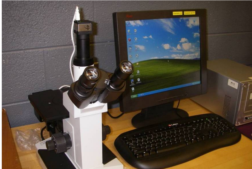
Figure 3.3: Photograph of Buehler Metallograph used to take pictures of 1018 steel and the Canyon Diablo meteorite. The specimens were etched using 7% nitric acid in Methanol and viewed using a magnification factor of 200x. The software used to view the images was U-Eye by IDS Corporation.
