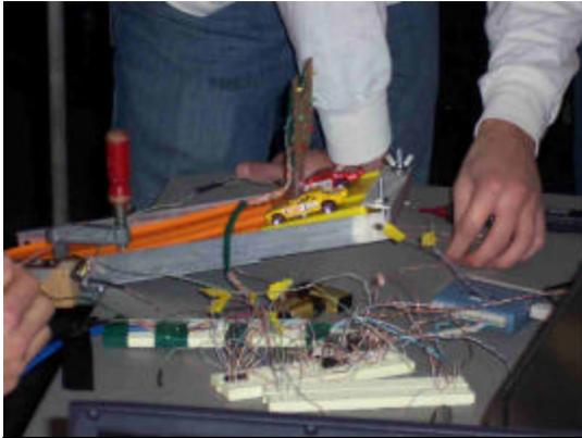
**Figure 1. Release mechanism, electronics, and digital IO board.**
