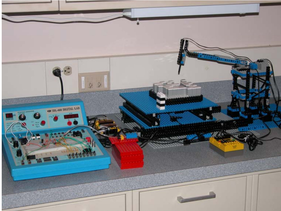
Figure 1: Complete Lego RCX-controlled model of IBM Millipede data storage device. On the left is the IDL-800 breadboard system, in the center is the X-Y stage on which sits the digital “data” under measurement, and on the right is the cantilever, or “arm.” A timer and shift register provide a bi-phase coded initialization signal to the X-Y stage RCX via a plastic optical fiber. At the end of the cantilever is the tip connected to a touch sensor. When the arm moves down, a rotation sensor provides information about the height of the bit.
