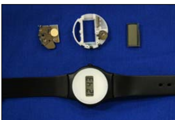
Figure 3: Internal components (top) and assembled liquid crystal display watch (bottom).
