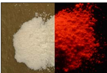
Figure 2: Nanocrystalline phosphor viewed under room light (left) and ultraviolet light (right).
