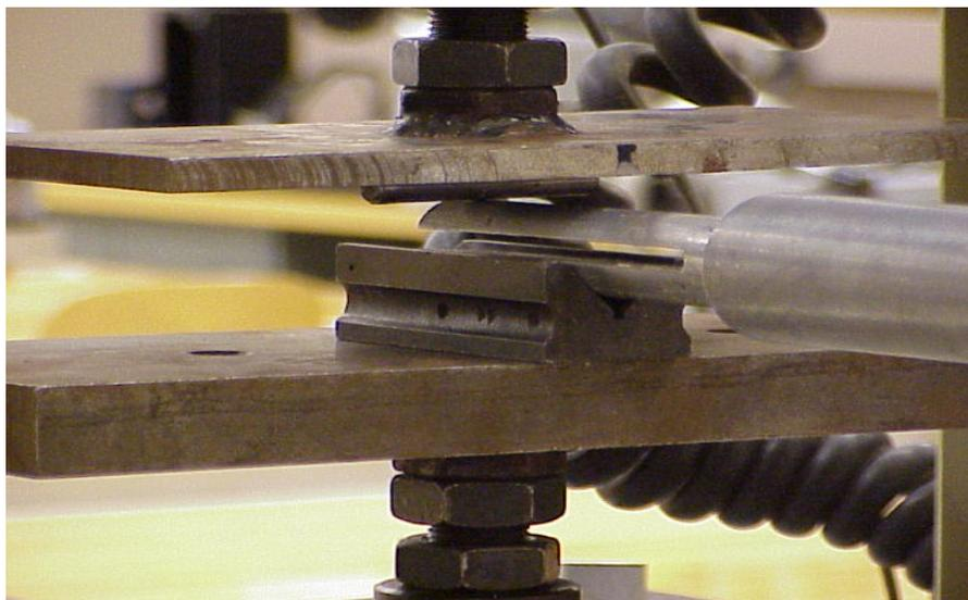
Figure 4: Fixturing to simulate wolf's teeth.
