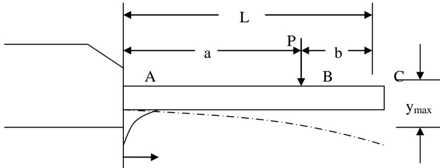
Figure 1: Cantilever beam (Mott, 2002).
