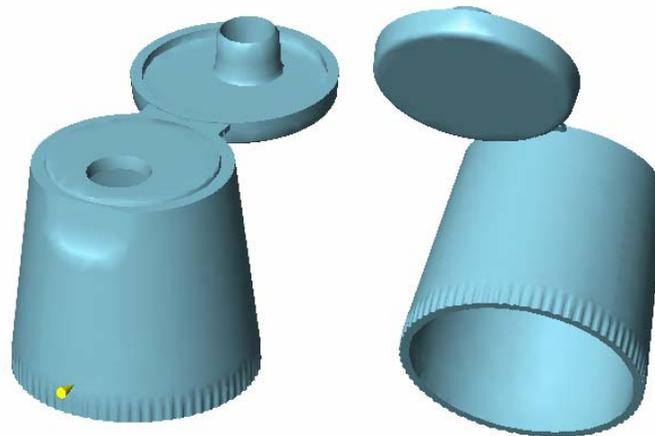
Figure 2: Solid model of 38 mm dispensing closure.
