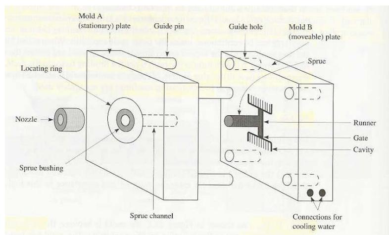
Figure 1: Typical plastics injection mold (Strong, 2000).
