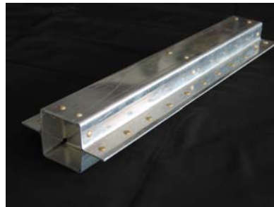
Two channels riveted together to form box beam
