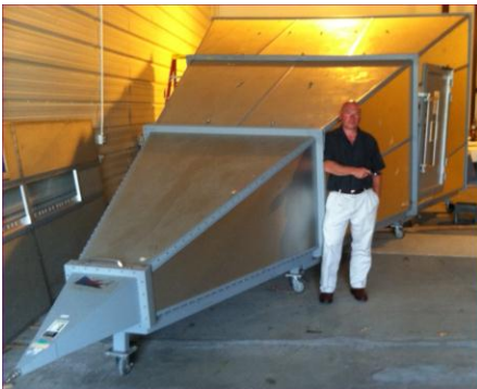
Figure 3.2 GTEM Cell for radiated immunity and radiated emissions
