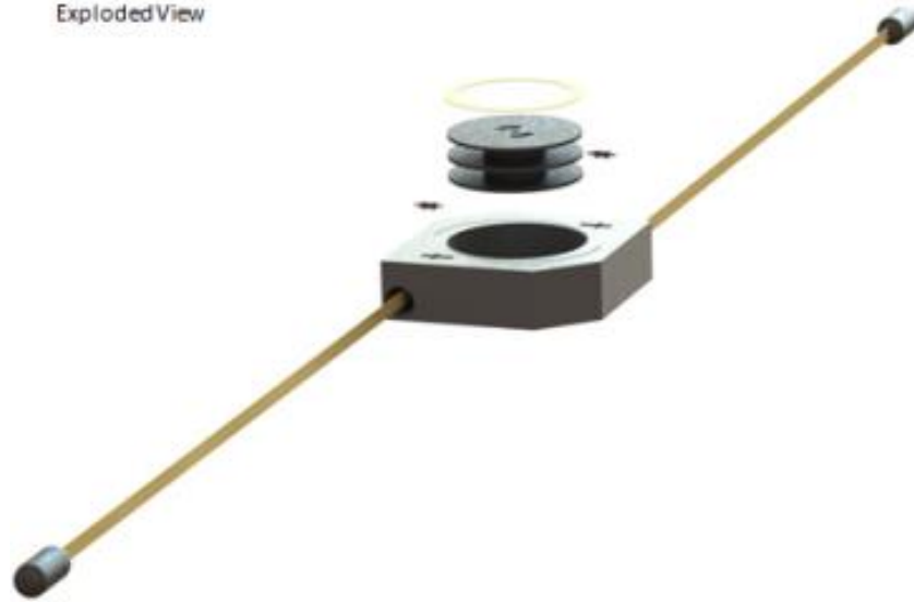
Figure 6. Exploded view of the boom system with VLF sensors.
