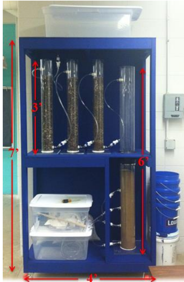
Figure 2. The built multimedia filtration system. The raw river water was stored in the plastic container at the top of the shelf to feed the system by gravity flow. The unit of the dimension is in foot.
